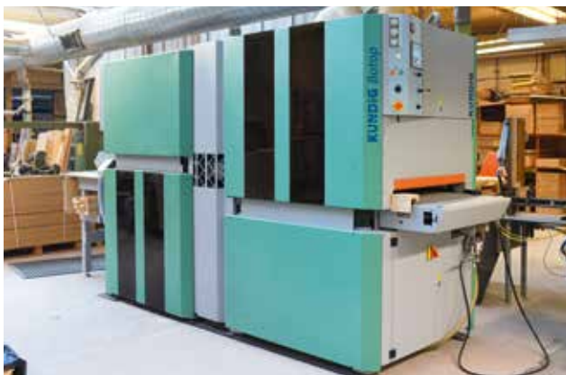
Overall six sanding-heads enable double-sided sanding with the Kündig Technic Botop-6 650-RRR-RRR.
