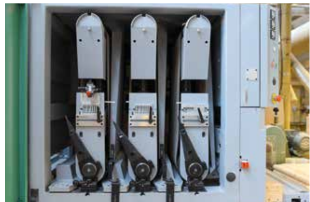
Equipped with three different grit-sizes it is possible to process parts from a planed surface to a finished surface in only one pass.
