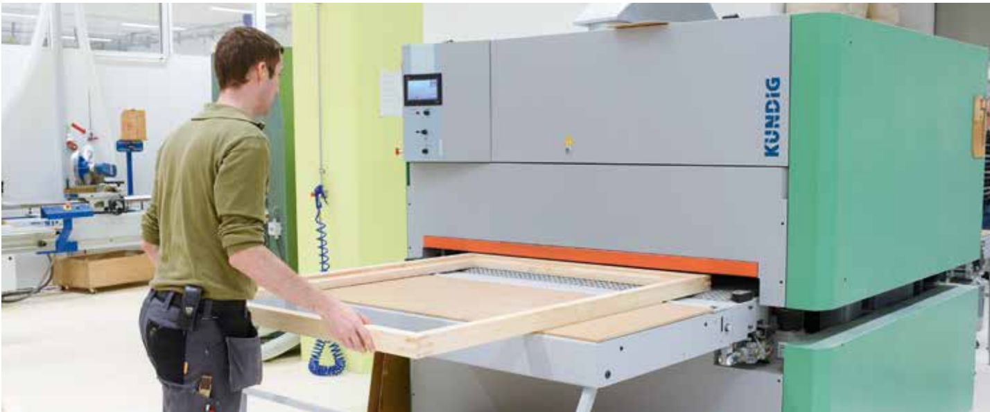
Window-sashes can be processed by the Kündig Brilliant-2 1600-RdPd-F with a standard working width of 1600 mm straight-forward. A special sanding-process enables perfect surfaces.
