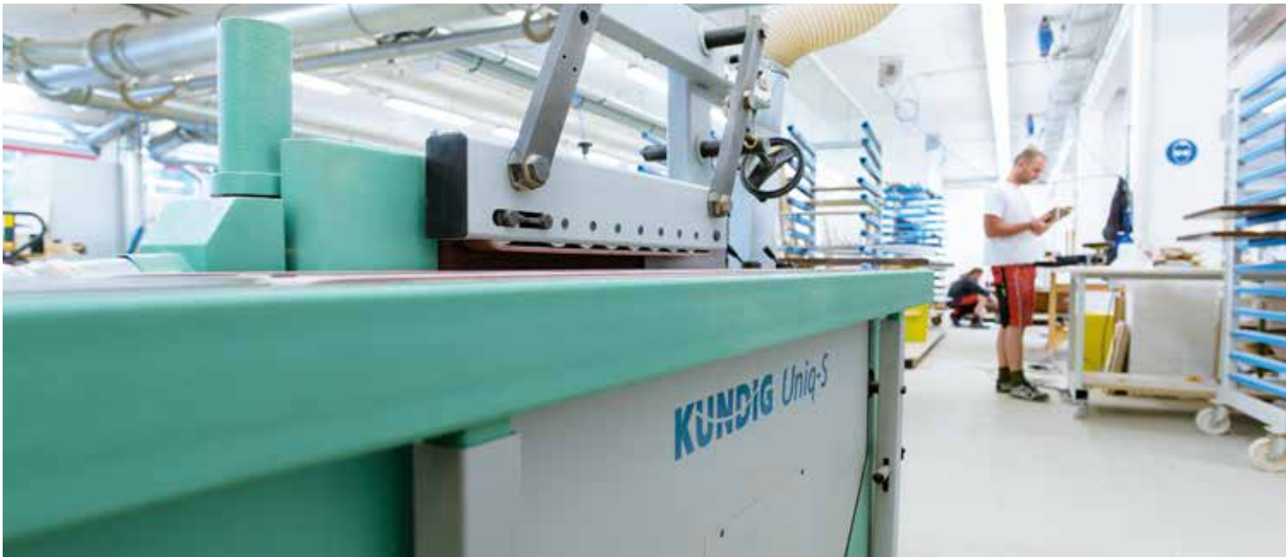
Overall three feeding-belts provide a gentle feed for delicate high-gloss parts with the Kündig Uniq-S Lack. Feed- and cutting-speed has stepless adjustment to the characteristics of applied lacquer-materials.
