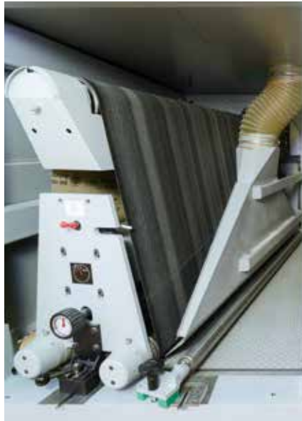
The two sanding-units form a "V" with angles of 350° and 10°. Sashes can be fed straightforward to make use of the whole working-width.
