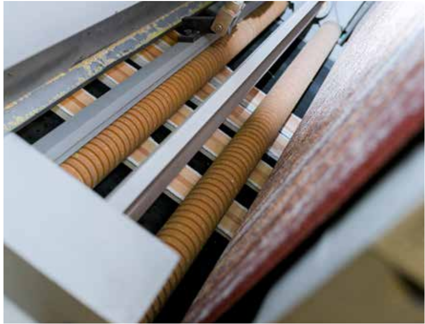
The sanding-head moves up- and downwards during sanding controlled by a computer and can grind up to 16 mm at one go. A vacuum feed belt keeps the ski securely in position.
