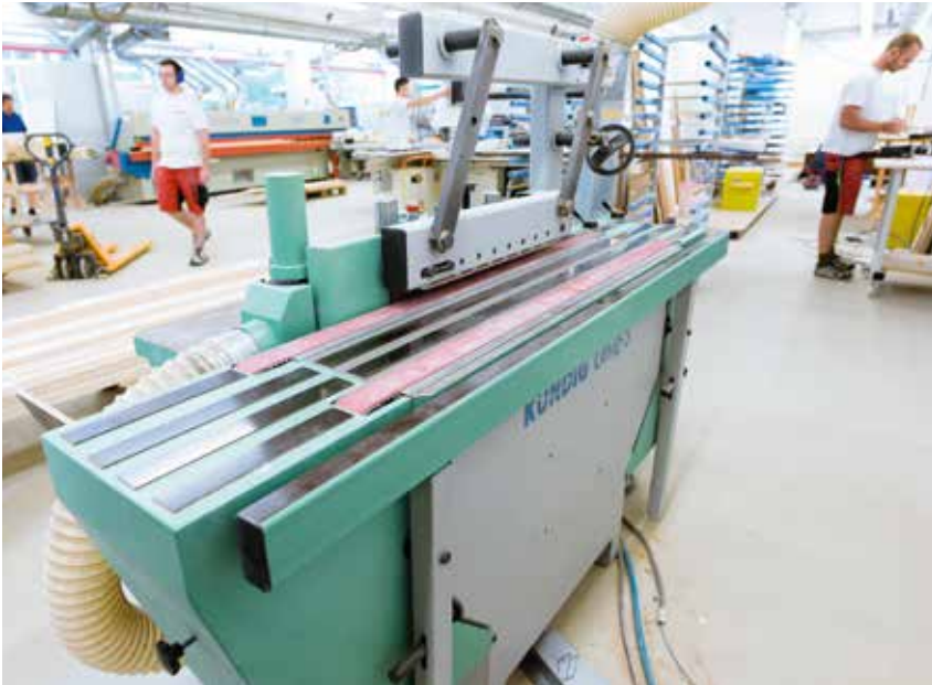
There are only a few edge sanders suitable for lacquer-sanding. Kündig's Uniq-S Lack enables this sensitive work to a very high standard.
