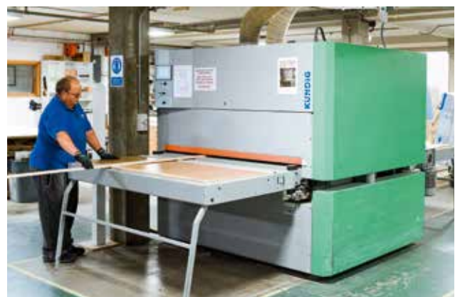
With a working width of 1600mm this Kündig Brilliant-2 1600-RCd proves to be a flexible addition to the large Botop sander.
